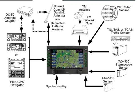
The FlightMax EX500 presents navigation, radar, datalink weather, lightning, traffic, and terrain data in an easy-to-interpret format, dramatically improving situational awareness and enhancing safety through all phases of flight.
